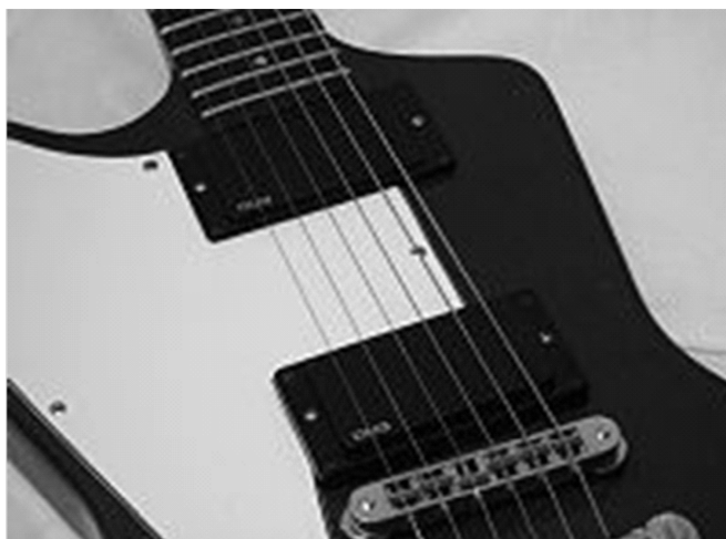
Fig. 1.5 EMG 81 and EMG 85 pair of popular active pickups
